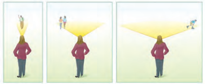
Figure 2. Examples of three settings of a hearing aid with adjustable directional beam widths. From left to right shows Narrow, Medium and Wide correspond to listening scopes of approximately +/- 50, 70, and 90 degrees, respectively.
