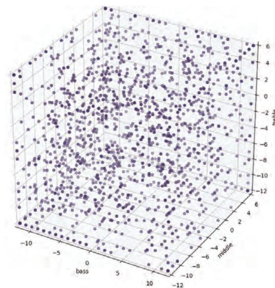
**Figure 2. SSL adjustments in the three frequency bands in a sample of 1,860 personal programs (Balling et al. 2019). Each dot represents a unique program; darker colors indicate overlapping programs**
