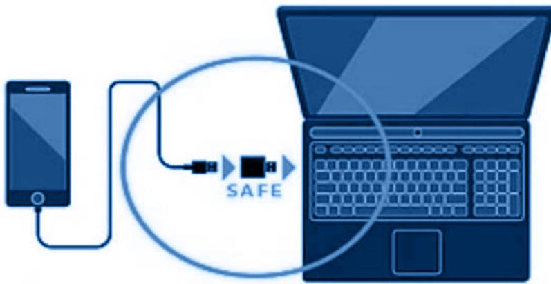
Figure 1. Prevent unwanted data access with a USB data blocker when charging a phone.
